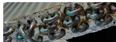
Copper tube and galvanized tube sheet after 500 hour salt spray.
